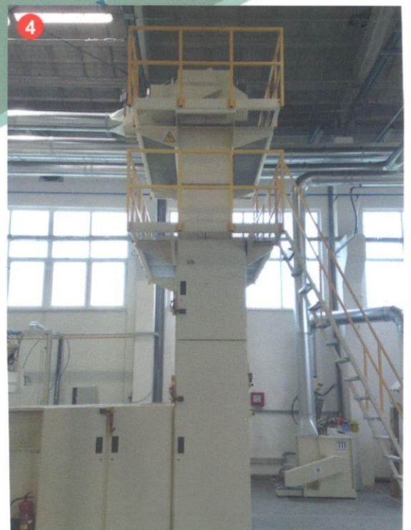
AUTOLEVELER HOPPER FEEDER MODEL CNA WITH CONTINUOUS WEIGHING CONTROL
